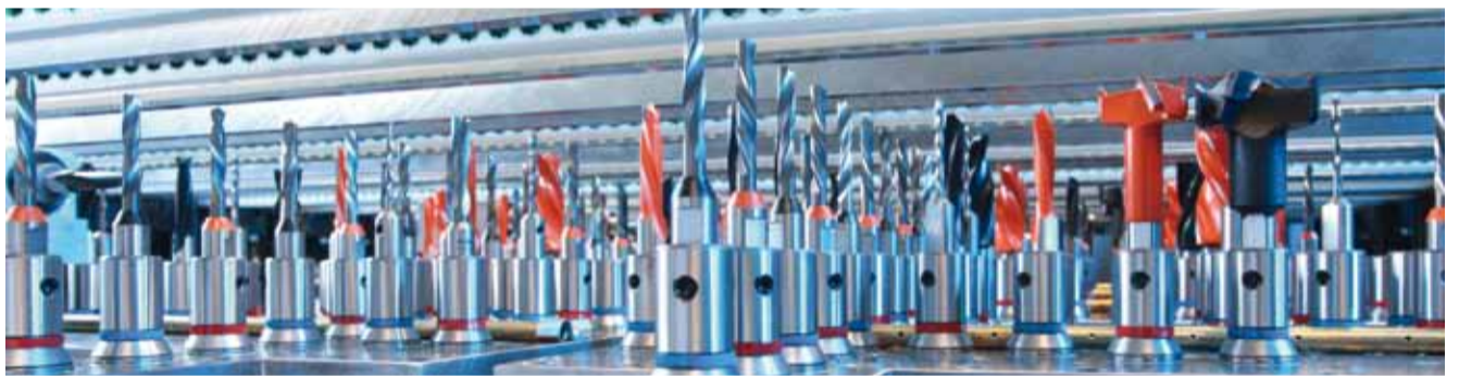
Throughfeed drilling for highly complex drilling patterns with small to minimal batch sizes
