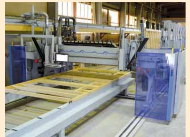
Production of timber frame element with the compactPLUS
