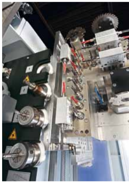
Vertical processing center: A single drilling gear with a total of 25 high-speed drilling spindles
