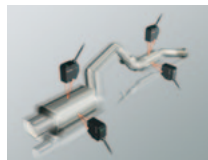
Vibration test of high-temperature-muffler
