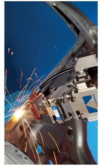
The laser welding is performed on many types of material, sometimes using pure argon or mixed, and in many other cases, using nitrogen. Nitrogen plays a very important role in laser welding applications on noble materials, among these are austenitic stainless steels, ferritic stainless steels and austenitic-ferritic steels (Duplex).
