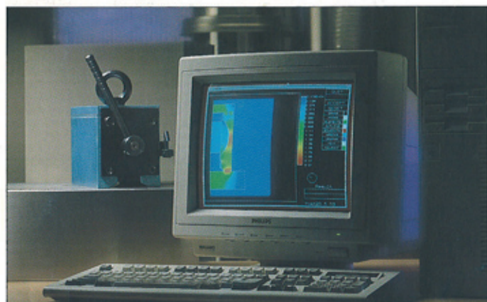
Calculation using finite elements for permanent lifting magnet
