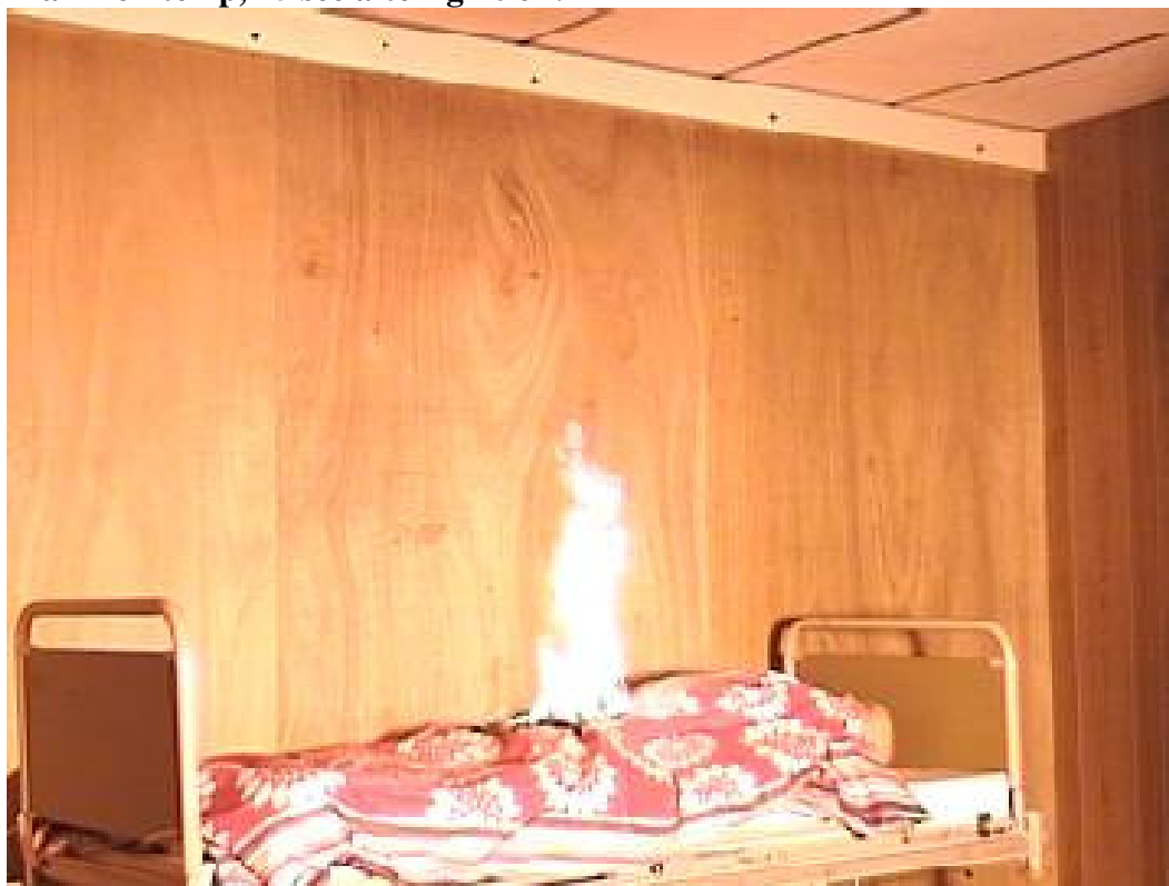
Alarm on temp, 25 sec after ignition:
