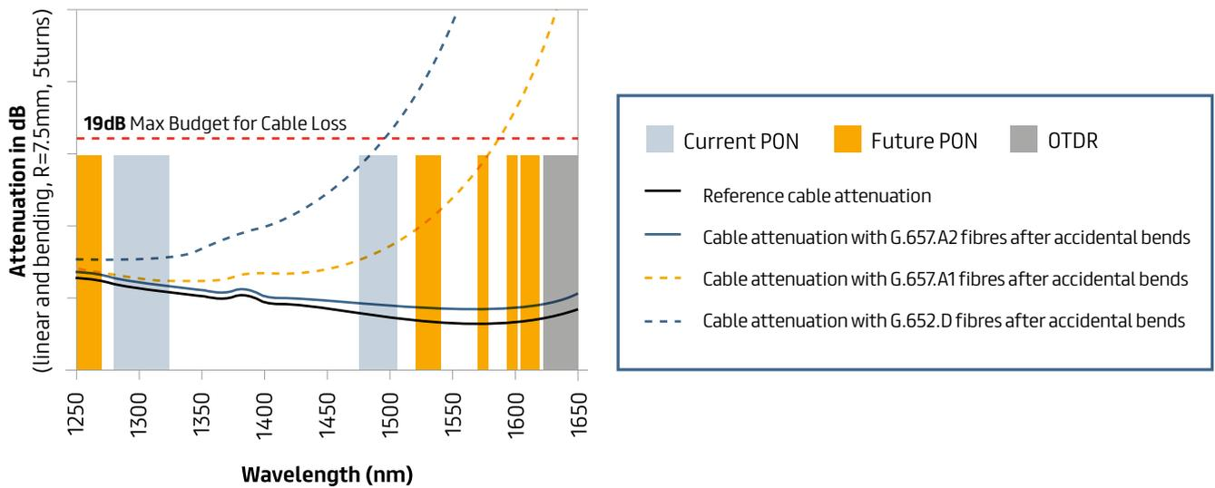
The above graphic demonstrates the attenuations which occur in an 18 km link over time, beginning on day one of access network deployment, and after accidental bends occur during the life-time of the network.
