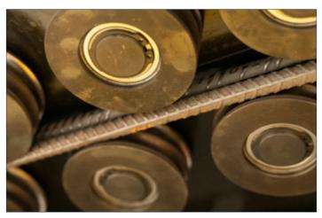
Straightening wheels are produced by most quality material with heat treated. It makes the machine firstly then parts very agile.
