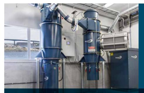
Dustcontrol supplies filter units designed to be installed in Zone 22 according to ATEX Directives 2014/34/EU.
