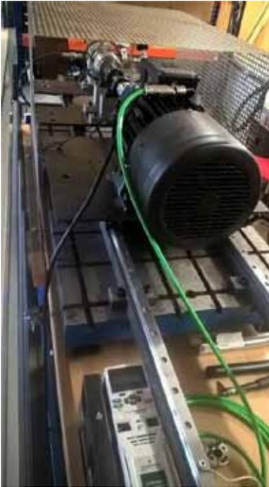
Test machine up to 150Nm.
