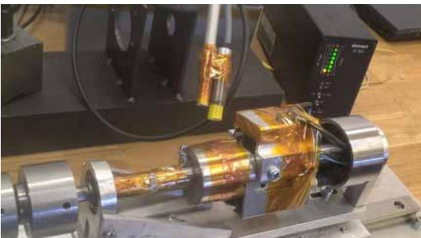
Test unit for testing our coupling for 0.001-10Nm.
