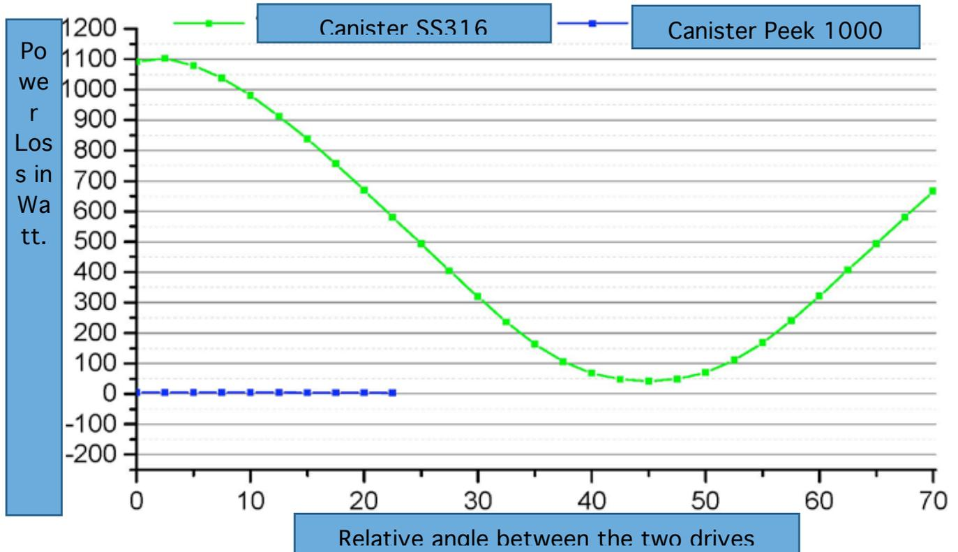
The table above shows the power loss at 1800 RPM with non-slip and under maximum work load.
