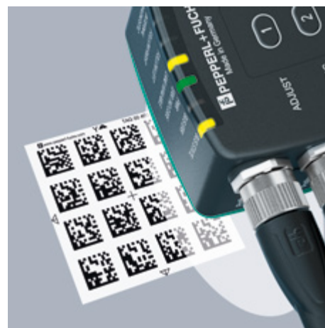
Grid navigation on Data Matrix tags.
