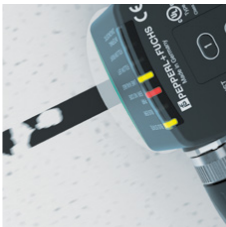
Seamless evaluation of damaged or dirty tracks.
