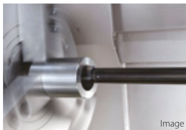
Image KAV-G20-10D / KAVH20-SCLCR09 CCMT09T304PP Overhang length: 140 mm (7D) / 200 mm (10D) Workpiece: SCM435
