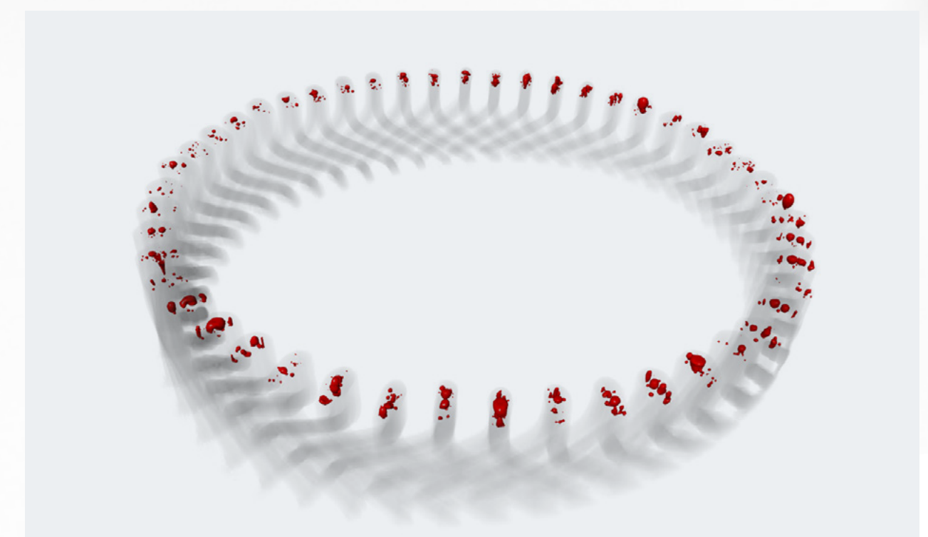
AI-supported, automated defect detection in the hairpins with ZEISS Automated Defect Detection (ZADD)
