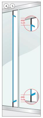
4. Remove approximately 5cm of the Liner at the bottom and the top and turn it to the back side.
