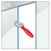
Pressure is essential for good adhesion performance and to avoid air bubbles. For optimal results we recommend a uniform pressure during application e.g. by a pressure roller.
