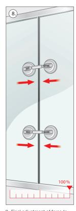
8. Final adjustment of force to reach optimal bonding results of both glass edges.
