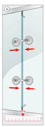
Join the glass panels together by using medium force of the vacuum device before removing the liner.
