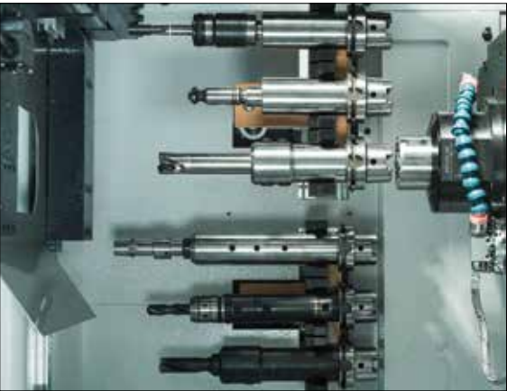
Automatic tool changer with 6 positions
