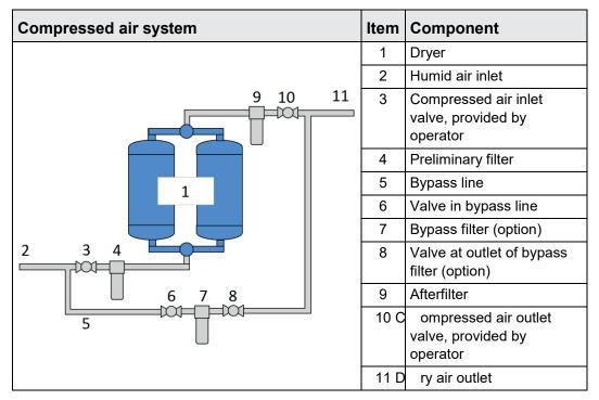
Example of proper installation with preliminary filter, after filter and bypass line.
