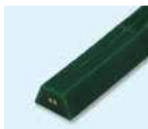
Result after overlap welding
