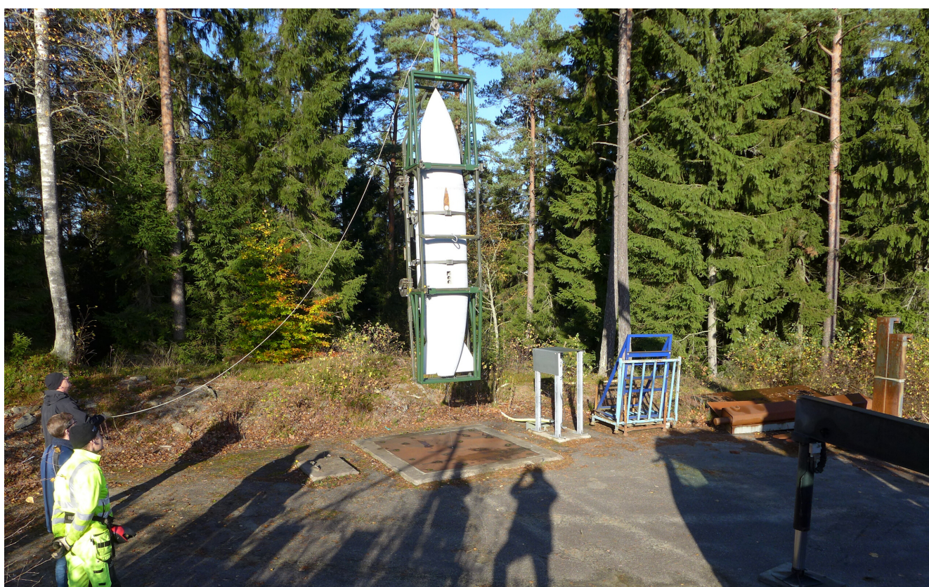
A drop test being conducted on Clip-Lok Steel Rack loaded a droptank in an external environment
