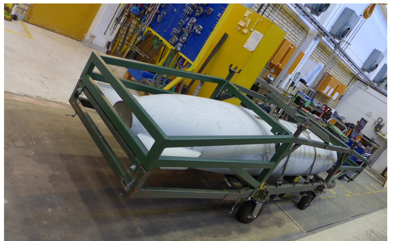
No damages or leaks detected in the droptank after the drop test was conducted by an internationally accredited test institute
