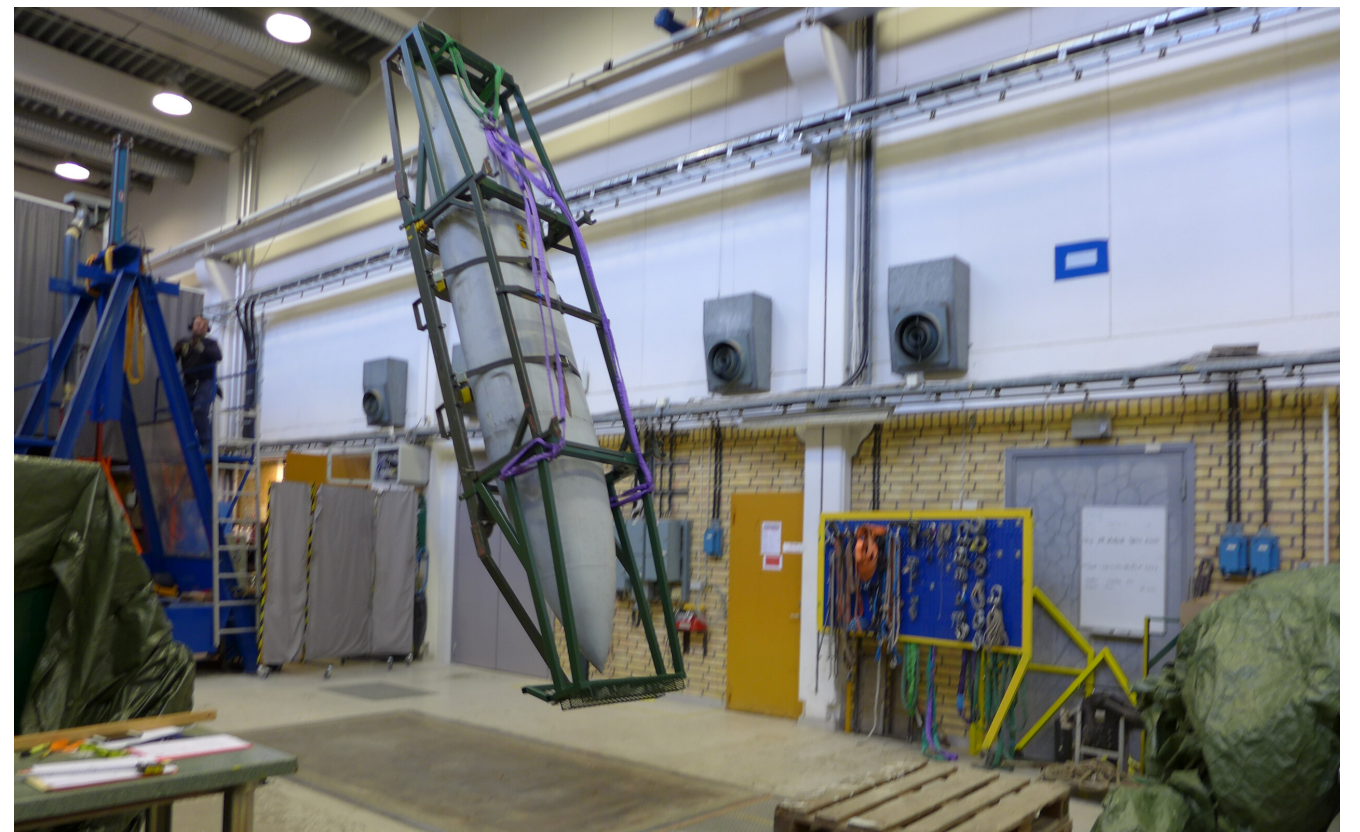
Clip-Lok Steel Rack loaded with droptank which is filled with aviation fuel is dropped from 1.2m as part of the drop test
