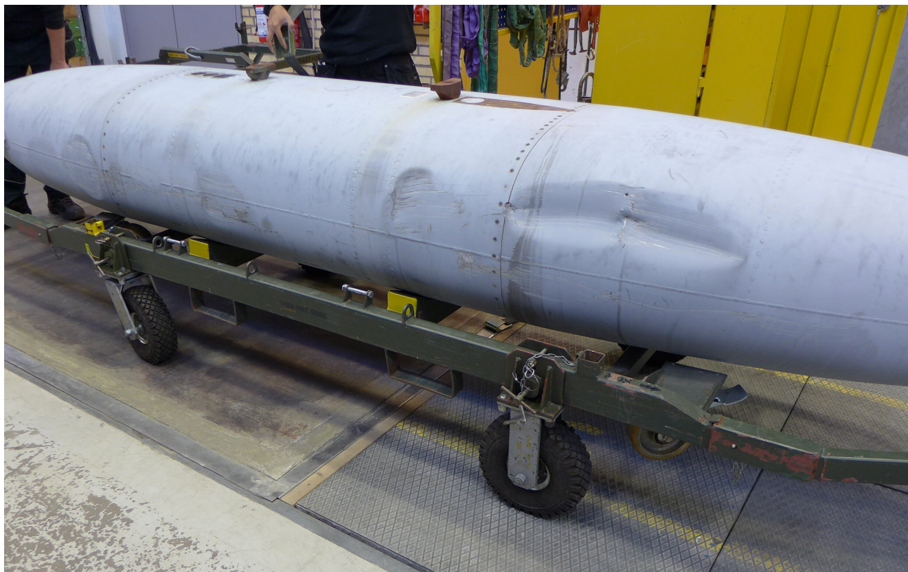
A droptank with aviation jet fuel brought on the existing under carriage ready to be mounted with Clip-Lok steel rack.
