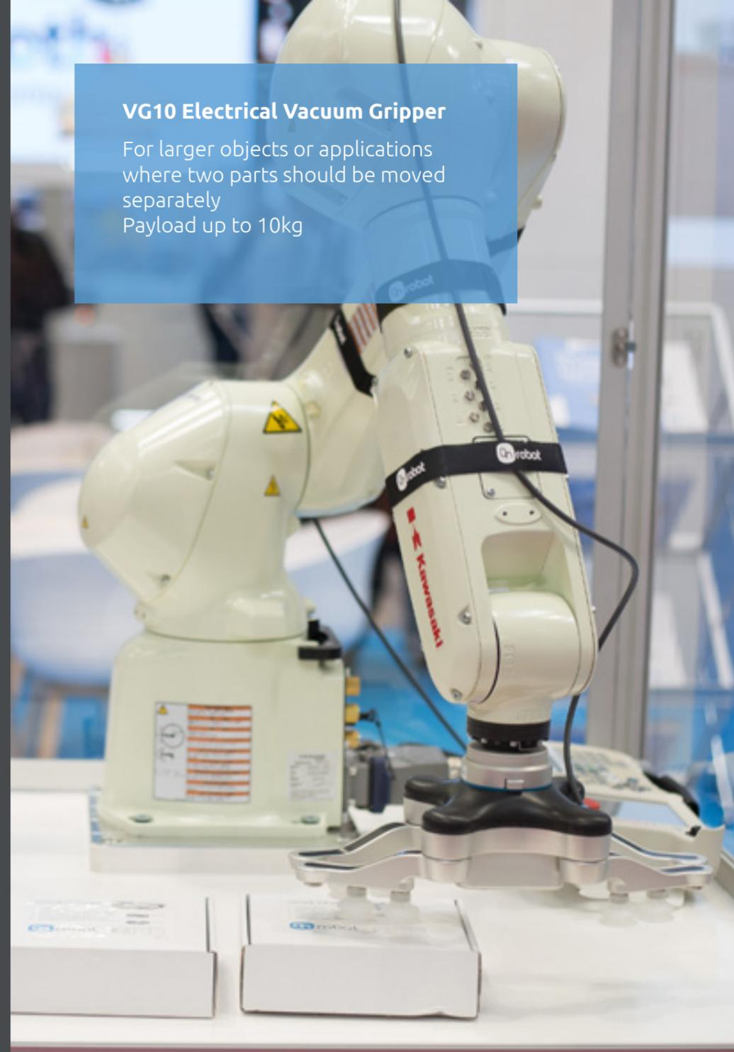
A photograph of the VG10 Electrical Vacuum Gripper robot arm. It is a white and blue dual-arm robot with 'Q robot' and 'KAWASAKI' branding. The gripper is a large, white, cylindrical vacuum-based device. The robot is mounted on a white base and is positioned over a white surface with some components.
