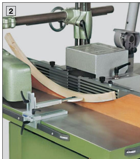
**1** Pressure module I and single wheel providing safe controlled pressure when edging curved workpieces.
