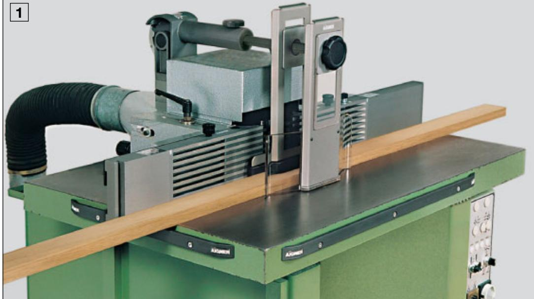
**1** Machining a narrow workpiece using a Centrex.
