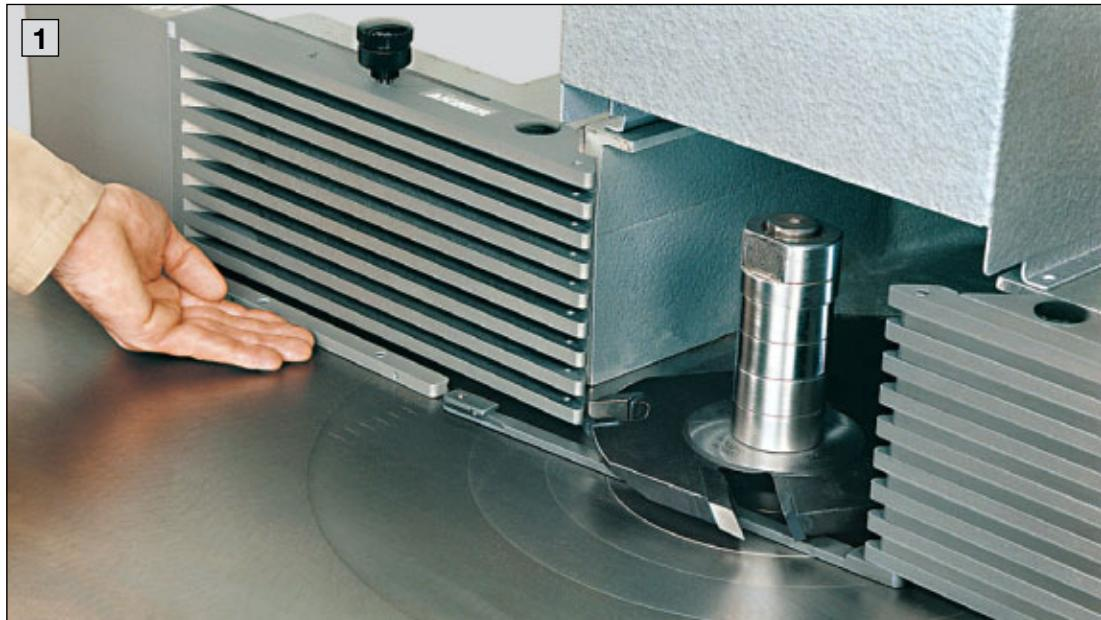
**1** Inserting the filling bar into the lower recess of the outfeed fence case.
