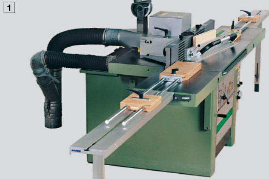
**1** Stop / drop on milling of short pieces using the clamp strip, variostop and table extension.
