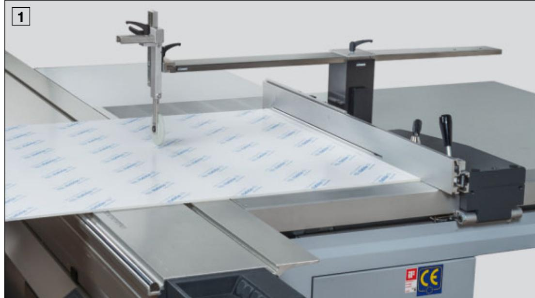
**1** Scratching an acrylic glass plate on the lower side using a pressure module □ and a single wheel.
