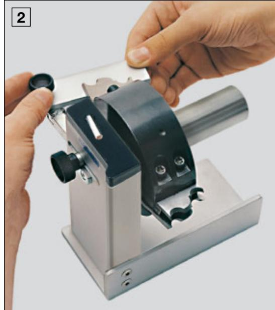
**1** Adjusting the marking plate to the machining cutter unit.
