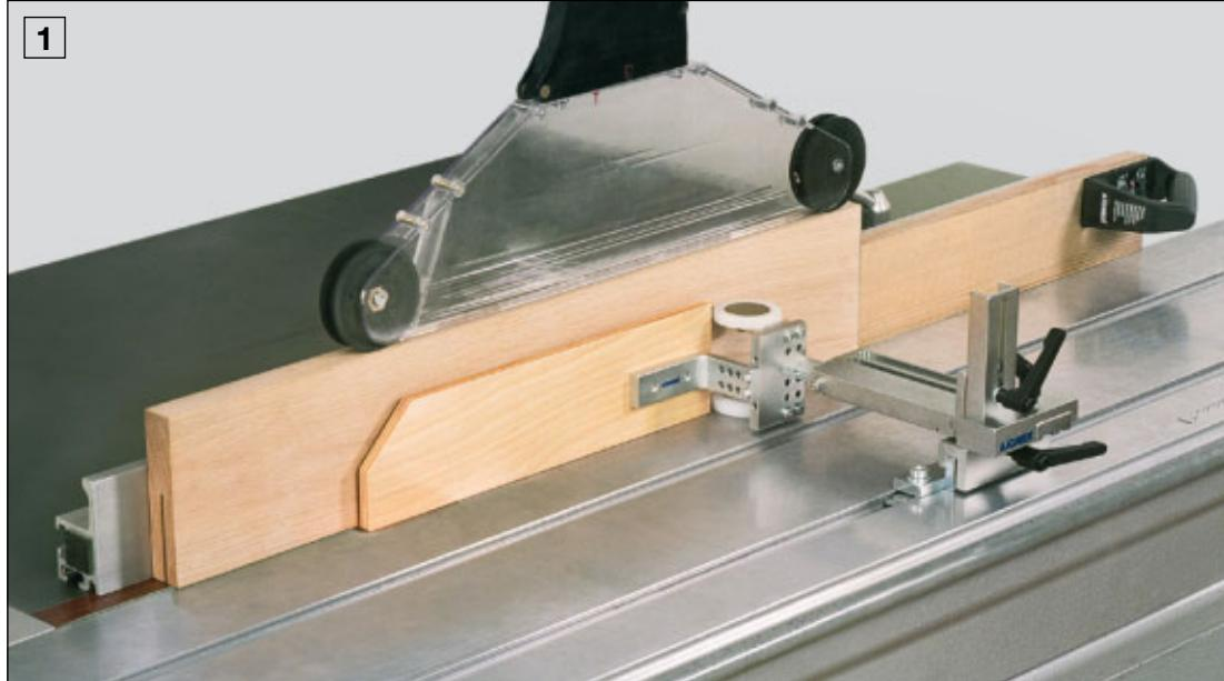
**1** Angle bracket with pressure module
