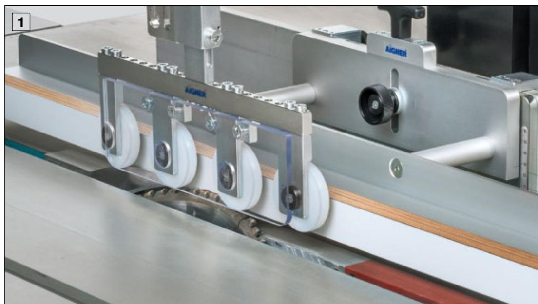
**1** Guiding ledge with protecting wheel. The saw blade is adjusted to the desired bevel cut.
