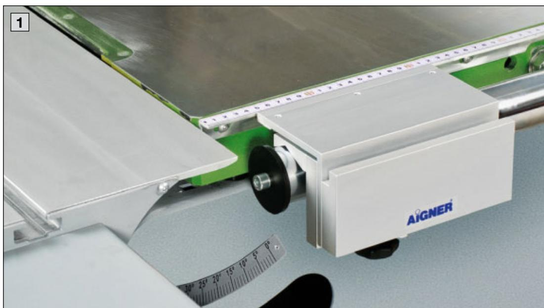
**1** Mounting adapter
