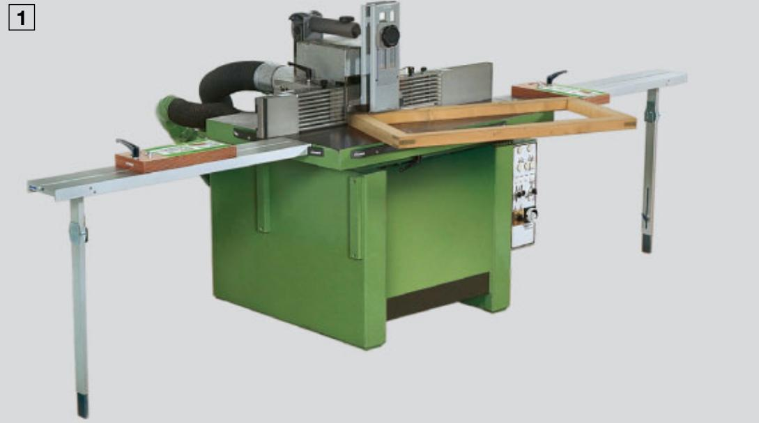
**1** Clips attached to the legs of both table extensions providing storage for the cross stops.
