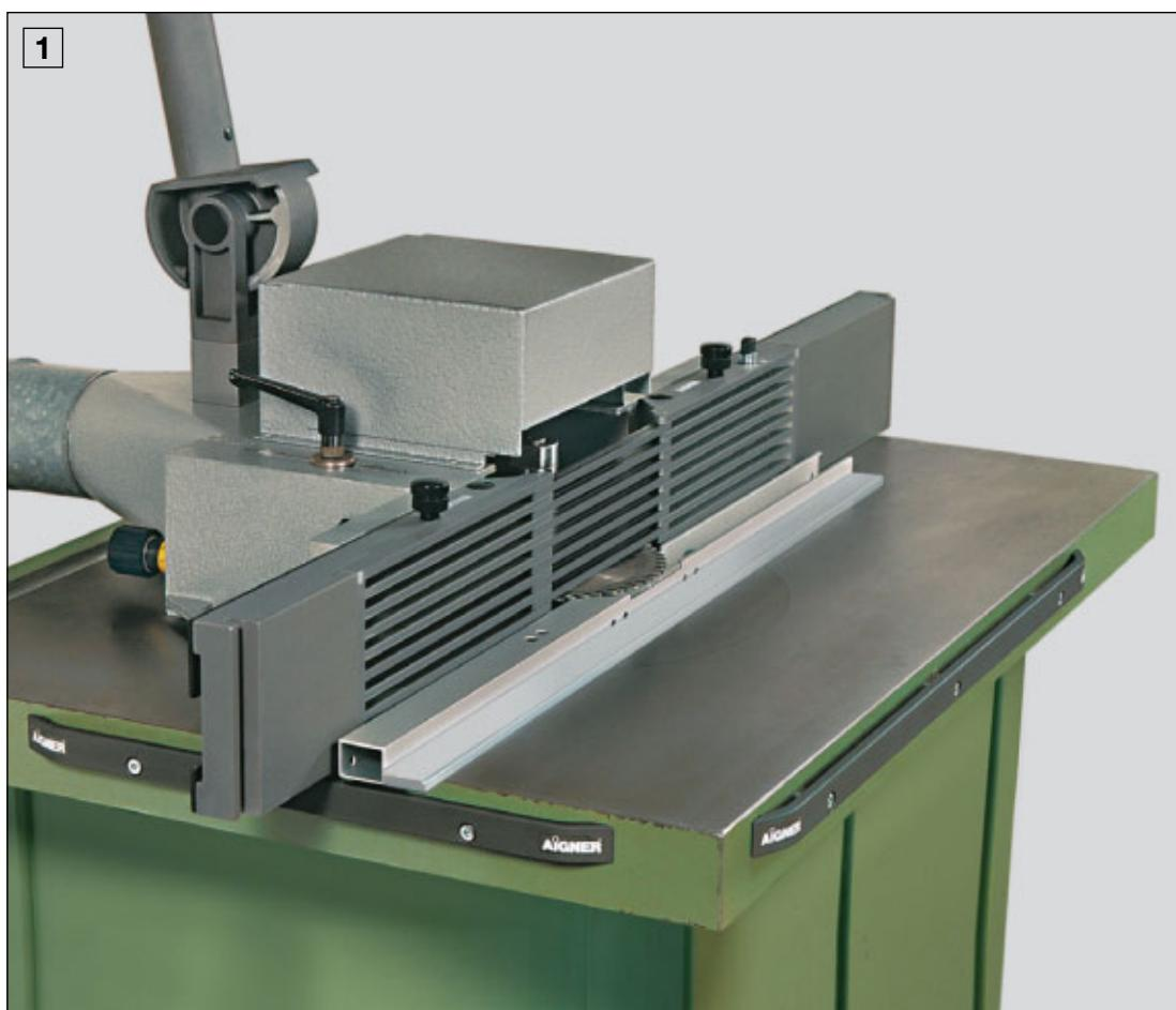
**1** Glassledger attached to the integral fence.
