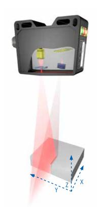
The laser line projected by the *PosCon3D* is reflected from the surface and depicted on a 2-dimensional optical receiver using the triangulation principle. The required optical image quality is ensured by the specially developed multilens system.
