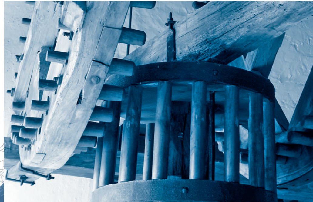
Traditional lantern gearhead in a mill: Technical template for the gearhead technology of EtaCrown®.
