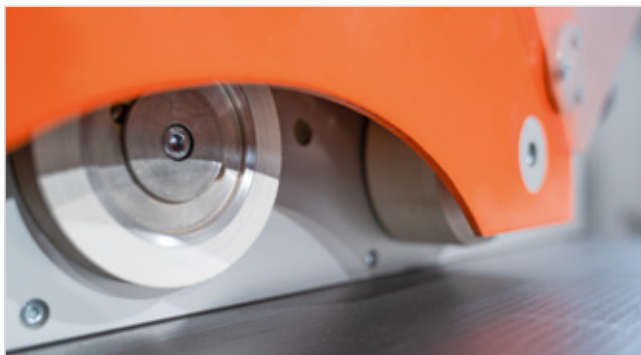
Circular saw power feeder 76: Feeding rollers in detail
