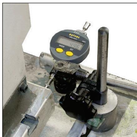
Measurement of the vertical displacement of an element
