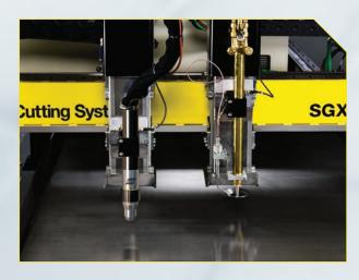
Equipped with up to three cutting stations, SGX gives you the choice of one plasma tool and up to two oxy-fuel tools.
