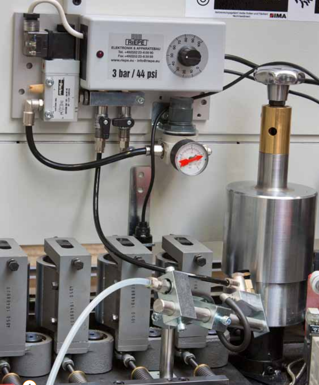
Installation example release agent spraying system for the pressure roller
