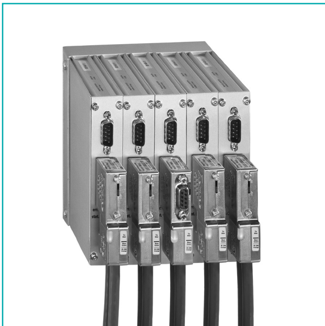
Bus connectors for PROFIBUS 90° with diagnostic LEDs
