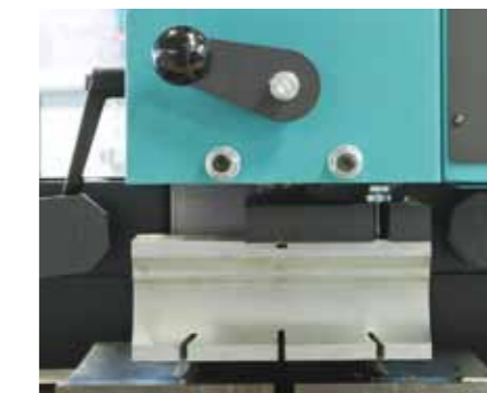
Short-stroke clamping cylinder with hand crank for pre-adjustment.
