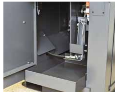
Big front door for good accessibility for saw blade changes and disposal of swarf.
