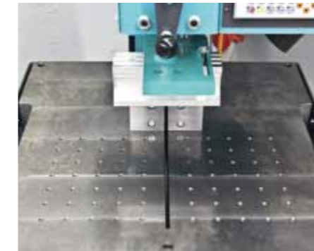
Drilling pattern in the saw table to enter fixtures of the customer's own design.
