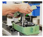
The DC-II gearbox is still manufactured in-house by Demag. This is the only way for us to meet our demanding quality requirement for the chain hoist.
