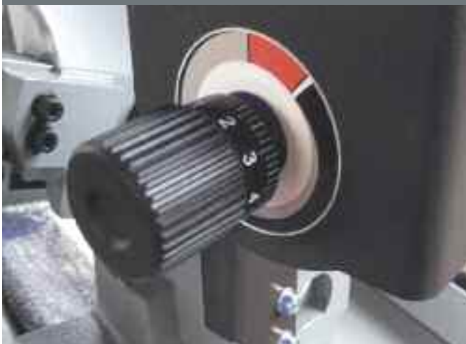
Convenient "push-pull" control knob for "Start and Stop" of the saw frame lowering (requires no modification of the preset lowering speed)
