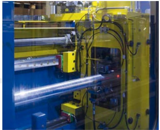
*Highest precision and maximum possible output are the main features of this peeling machine which has especially been developed for the peeling of aluminium bars.*
