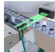
Measuring the outer diameter of connector housings
