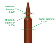
Measuring the outer diameter of ampoules
