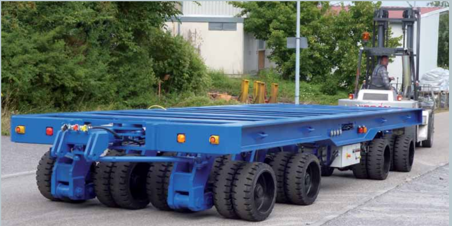
Heavy-duty trailer, 100 tons, type 70-8 HH with hydraulic lift
