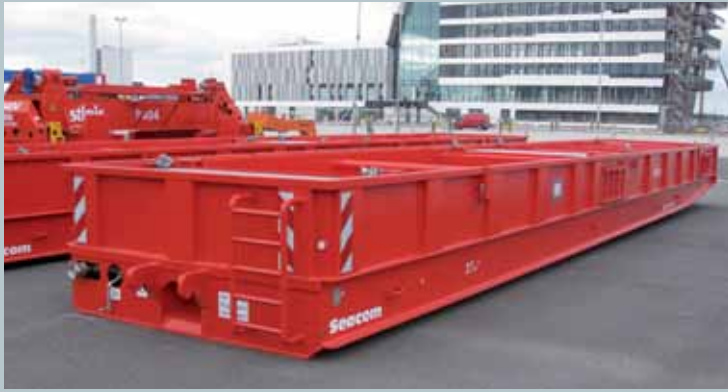
Roll trailer with 27 m 3 reservoir for leaking containers, 63 tons
