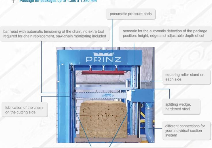
cutting equipment driven on both sides, moving on high rigid linear guideways direction of cut as requested: from top to bottom, bottom to top or in both directions, as DOUBLE ACTION
