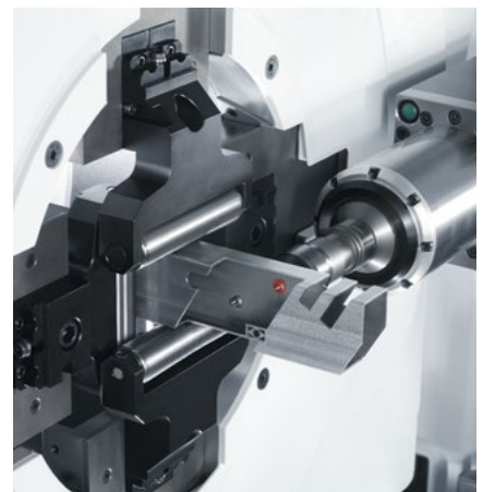
Threads can be created automatically, even in thin materials.
