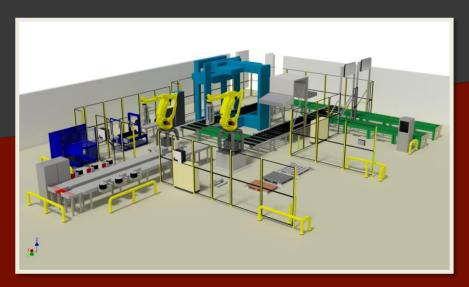
Full automated palletizing solution, that recognizes and depalletizes pallets from the warehouse and afterwards reads labels, prints and applies new labels before palletizing on to customer specific pallets. The solution uses state-of-the-art FANUC robots and vision systems, and provides advanced scanning and a unique gripper which is able to handle many different customer specific products.
