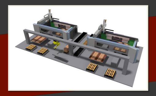
Fully automated processing in CNC-machines combined with fast gantry robot keeps the machines busy by keeping them loaded with raw material. The robot palletizes the finished products as well. The two tables at both machines reduce the waiting time for loading new material to process.
