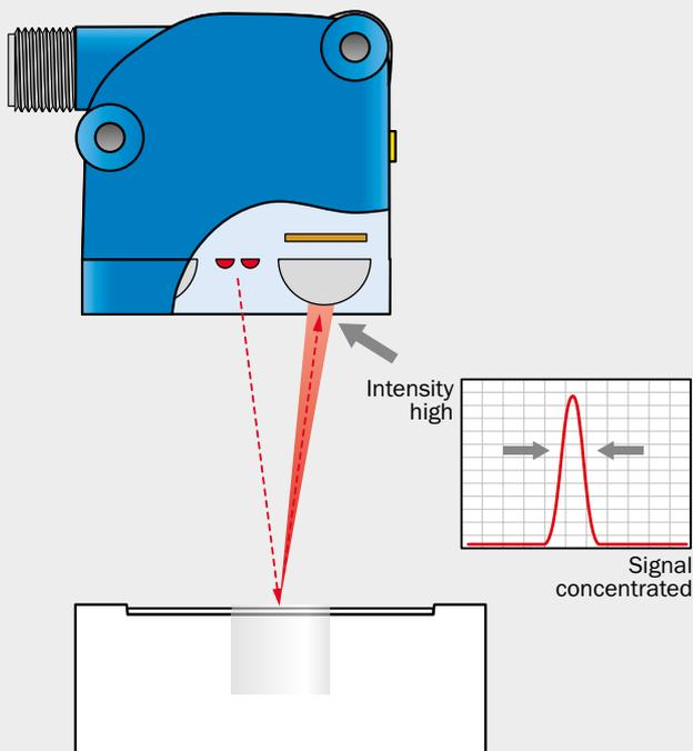
At a defined angle, visible red light lands on the object to be detected. Depending on the gloss level of the surface, the light beam is thrown back with a different intensity and scatter.
