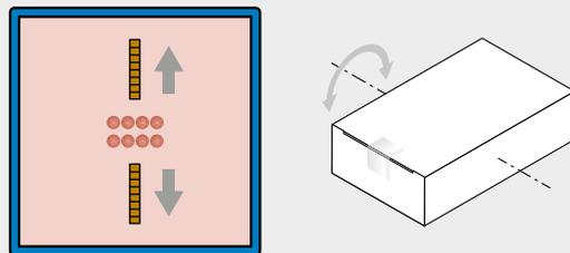
With receivers arranged vertically to the red-light LEDs, Glare is immune to vertical tilting.
