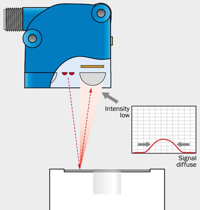
This information is recorded and analyzed via two high-resolution line sensors with the patented Delta-S-Technology.
