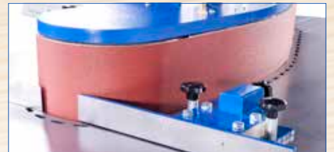
Veneer sanding unit and circumferential table extraction
