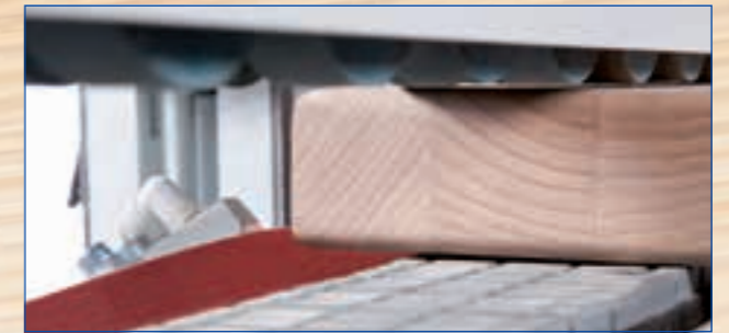
Profile sanding on top/bottom
