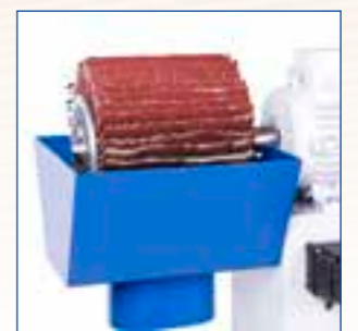
Sanding brush with adjustable extraction hood
