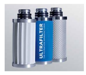
The secret of this vast increase in performance lies in the pleating of the nano-filter media. The pleating process mechanically folds the non-woven filter media many times. This makes the filter area 450% larger than that of a conventional rapped filter element.
