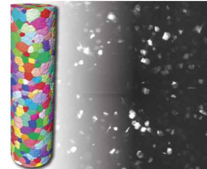
Crystal structure of an aluminium-copper alloy, used for example in aircraft construction due to its low specific weight
