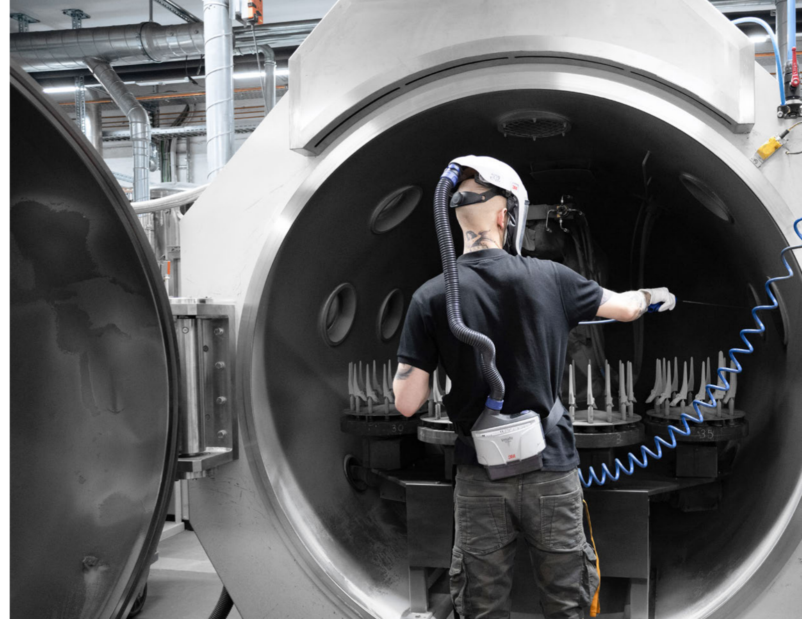
The prostheses are coated in the vacuum chamber at a temperature of up to 20,000 degrees Celsius
