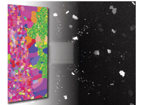
Crystal structure of an ultra thin oriented electrical steel sample, used for example in electric motors, transformers or generators
