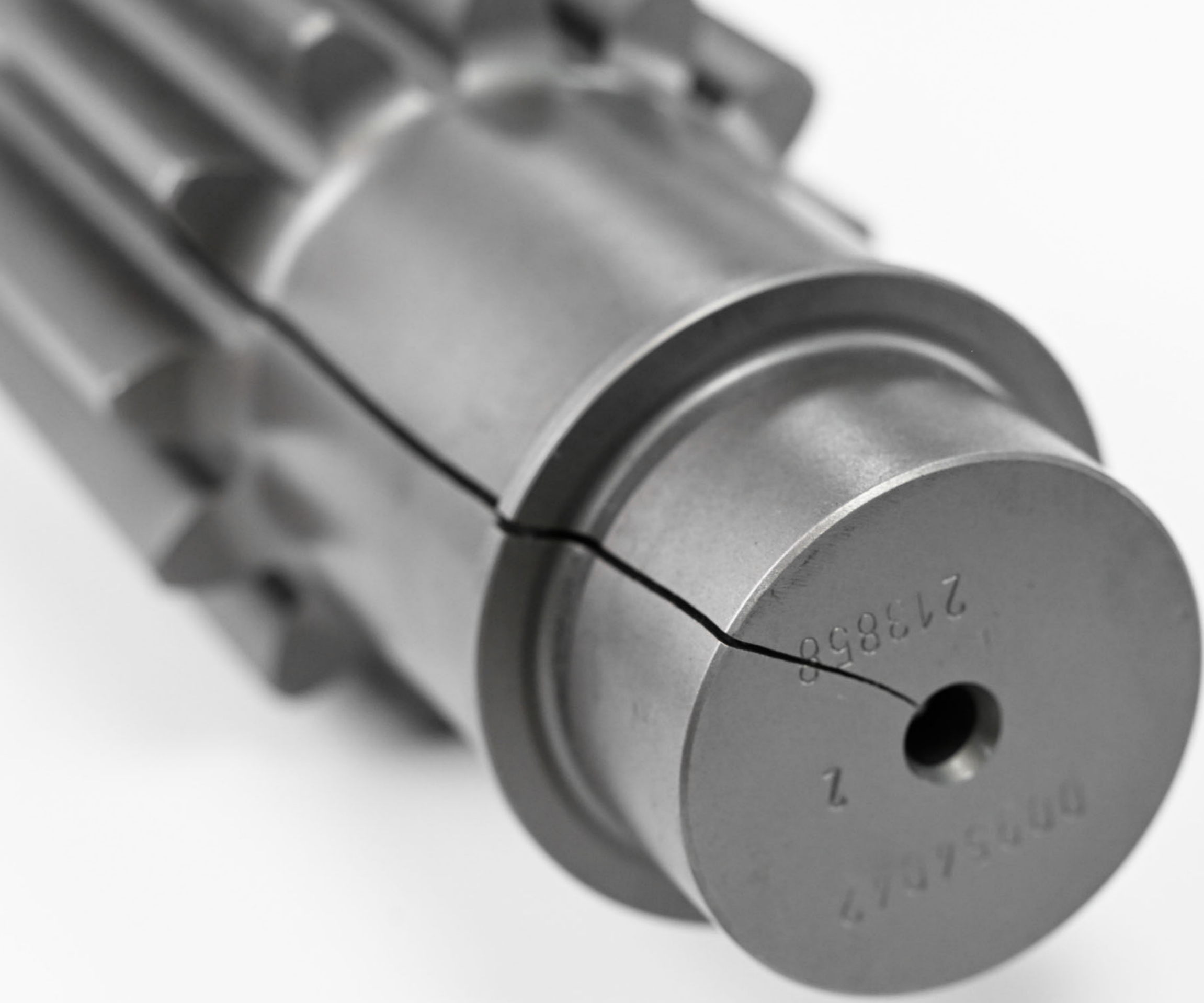
What caused the crack in the pinion shaft? The SPC materials laboratory determined the cause of the defect using ZEISS microscopy solutions
