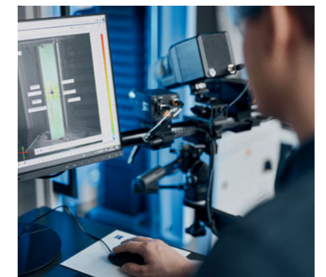
Recording the strain behaviour of a open hole tension specimen with ZEISS ARAMIS
