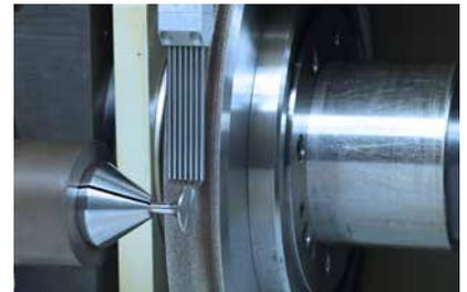
+ **Weight optimisation:** Through targeted material reduction at the core, weight reductions of up to 50 percent can be achieved. POLARIS LW tools determine less wear on spindles and bearings than comparable reference tools. Moreover, significant advantages arise during transport and fitting of the tools. A patent has been applied for with regard to this innovation.
