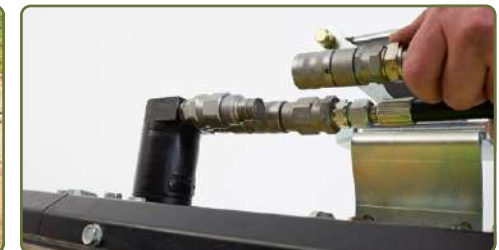
Hydraulisk snabbkoppling (standardutrustning).
