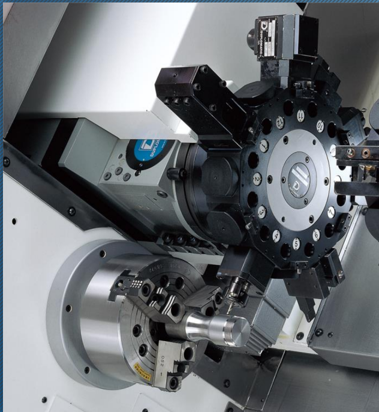
Main and counter spindle are running synchronous
