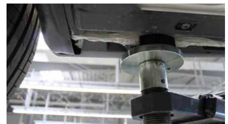
Form-fit support adapters to suit the vehicle type.
