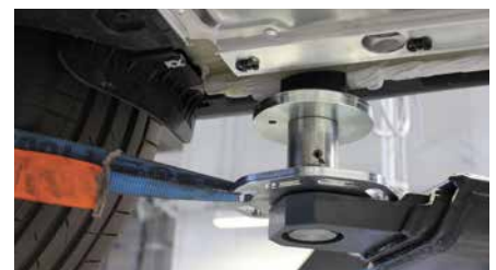
Vehicle securing system with lashing straps.
