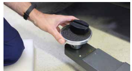
Support disc system (ATS) with plug-in system for swing arms or rubber discs (120 mm).
