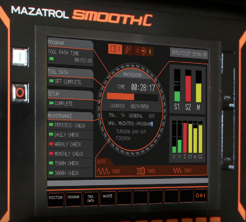
Process home screen The home screen displays overall process status in an easy to understand manner.
