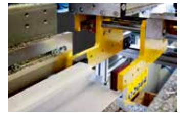
4 axis version available with saw blade 90° diam. 450 mm
