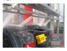
Especially developed for the touchless wash of the vehicle front and upper areas or to enhance cleaning results with demanding vehicle fleets. It works with 16 zero-angle nozzles at 70bar and 126L/min. and with an oscillation motor and a spinning motor for software-controlled 180° motion.
