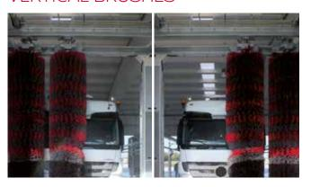
The self-driven vertical brushes perform an overlapping scrub on the vehicle front and rear. Brush positions are controlled by means of an encoder and the brushes of high density polyethylene work with three pressure levels for the different vehicle shapes. Patented front tilting system –for improved cleaning results on the windscreen– is optional.
