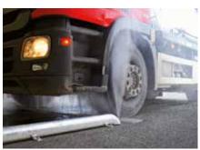
Drive-through underchassis wash with high-pressure, working at 70 bar and 126L/min. With entry photocells for an automatic operation and 12 rotating zero-angle nozzles, it is installed at the start of the bay. It can work with the same high-pressure pump rack that feeds the rollover by means of a solenoid valve.
