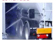
The perfect optional extra to complement the brush-wash process in lower vehicle areas or on corners inaccessible to the brushes such as rims, underside, or tanks. It consists of 16 zero-angle nozzles to operate at 70bar and with 84L/min. or 126L/min. It works with an oscillation motor (up-down) and a rotating cylinder (forward-backward) to thoroughly clean this area from different angles.
