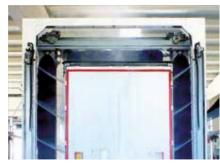
Recommended to thoroughly wash the upper side of the vehicle, particularly for tankers, garbage trucks or vehicles with special profiles, and to reach areas inaccessible to the vertical brushes. Consisting of 24 zero-angle nozzles to operate at 70bar and 126L/min., it works with an oscillation motor (up-down) and a rotating cylinder (forward-backward).
