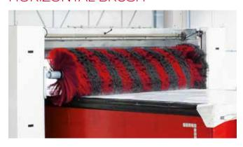
The high density polyethylene horizontal brush is equipped with a frequency converter to soften up and down movements, and with **5 pressure levels** to better follow vehicle profiles. Thanks to the model's flexible configuration, up to 4 'obstacle-avoidance' scans for wing mirrors and sunscreens are also possible.
