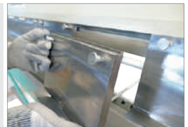
1 Quick disassembly of the segments with pull-device
