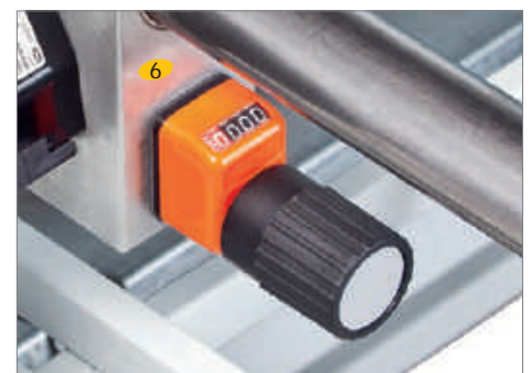
Back gauge conical adjustment
