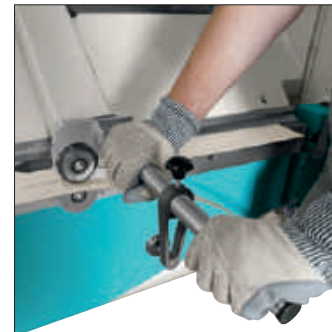
Retractable manual roller shear in cutting position, Ref. PTSL-CCM
