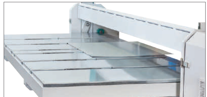
Electric back gauge, maximum range 750, 1000 or 1500mm - Ref. PTSL-BAE
