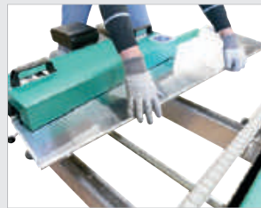
Roll-formed conical tray in 2 runs
