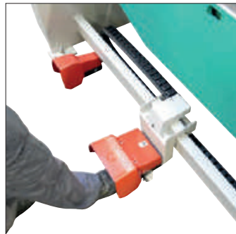
Control pedal on ground rail Ref. PTSL-PEDRAIL
