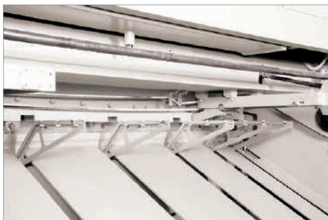
7 Pneumatic sheet holding plate
