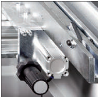
Pneumatic conical folding, manual adjustment
