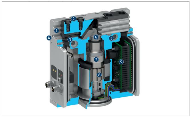
The brushless servomotor forces the wedge-hook up or down via a ball-and-screw spindle drive. Through its angled active surfaces, the wedge-hook transforms this motion into the horizontal, synchronous movement of the base jaws.
