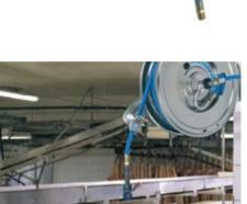
This hose reel, made entirely of stainless steel, is designed specifically for the food processing industry. It is very easy to clean thanks to rounded edges and features an easy to dismantle hose outlet, an externally mounted swivel, and a minimum number of material joints.
