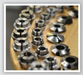
We work within these dimension areas: round rods 2–16 mm, hexagonal rods 3–8 mm and square rods 4–6 mm. Internal threads span the interval M1.4 – M14. Our ROTEX lathes have a maximum product diameter of 10 mm and our Citizen CNC turning machines have a maximum product diameter of 16 mm.
